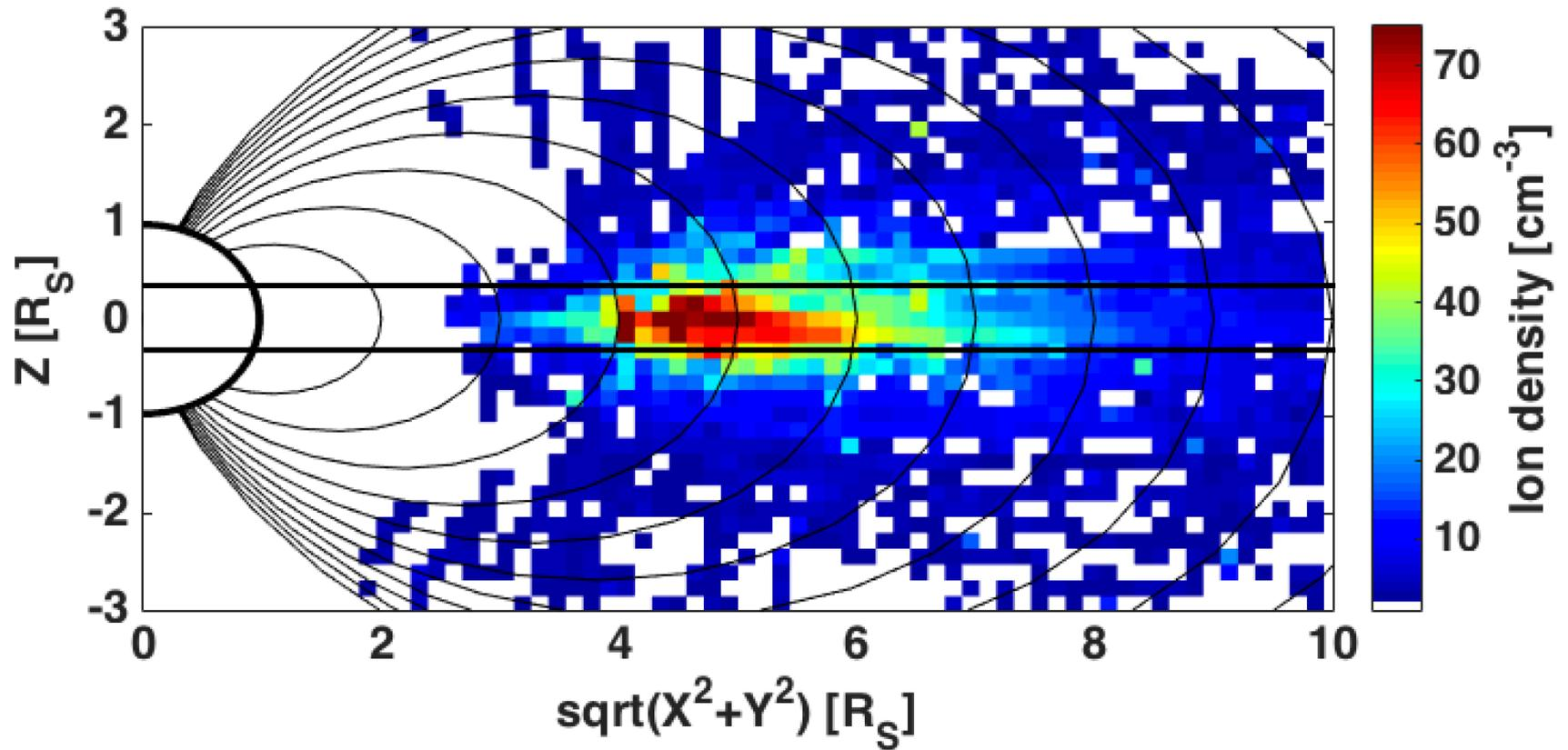
Figure 6. Average of ion density vs. distance from Saturn, magnetic L shells (black lines) 2 to 11. Bin size 0.15 in r and z.
