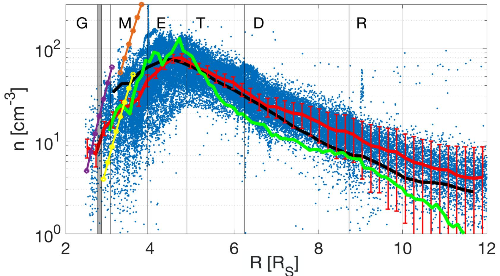
Figure 7. Equatorial,  $|z| < 0.25 R_S$ , ion densities (blue dots). Median LP ion density (red) for each  $0.2 R_S$  radial bin, median electron density from upper hybrid resonance (UHR) frequency measurements (black), CAPS ion density (green) (Livi et al., 2014), CAPS ion density for years 2007 (purple line with circular markers), 2010 (yellow line with markers), and 2012 (orange line with markers) (Elrod et al., 2014)
