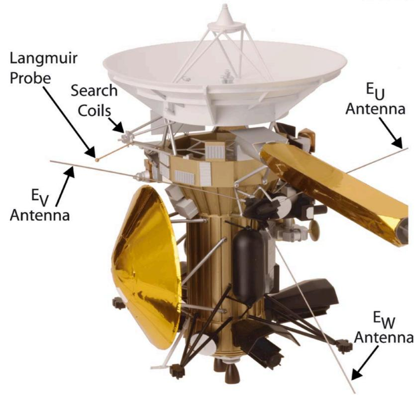
Figure 3: Cassini and the Langmuir probe. Image from Gurnett et al., 2004.
