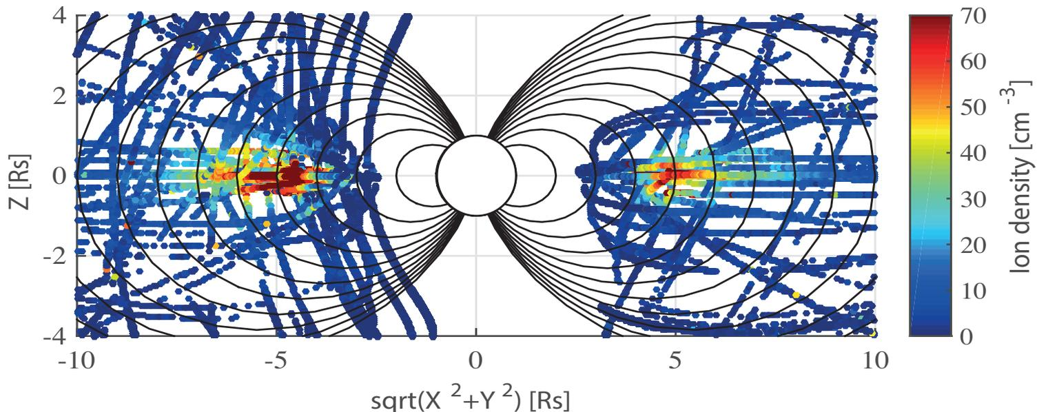
Figure 5: Ion densities derived from Langmuir probe measurements, showing the extension of the inner plasma disk.
